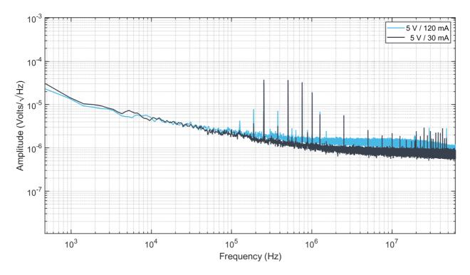
$<sup>^{25}</sup>$  RMS noise measurements are bandlimited to 50 MHz and are done at full power supply load.
